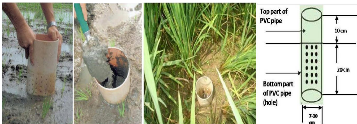
Figure 2: AWD device installed in the soil.
