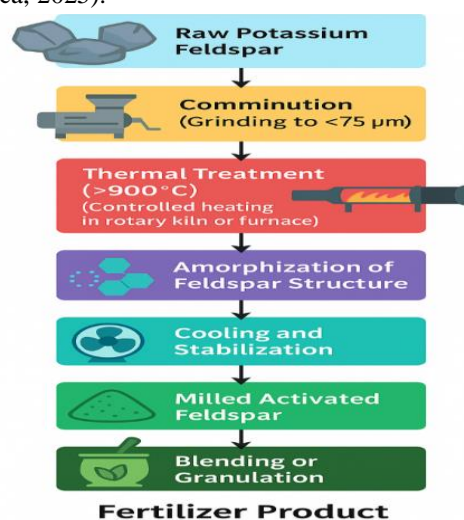
Figure 3. Thermal activation flowchart for potassium feldspar in a rotary kiln or muffle furnace (900–1150 °C, 30–90 min residence time). The process involves grinding (<75 µm), heating under a controlled atmosphere, cooling, and post-milling prior to granulation.
