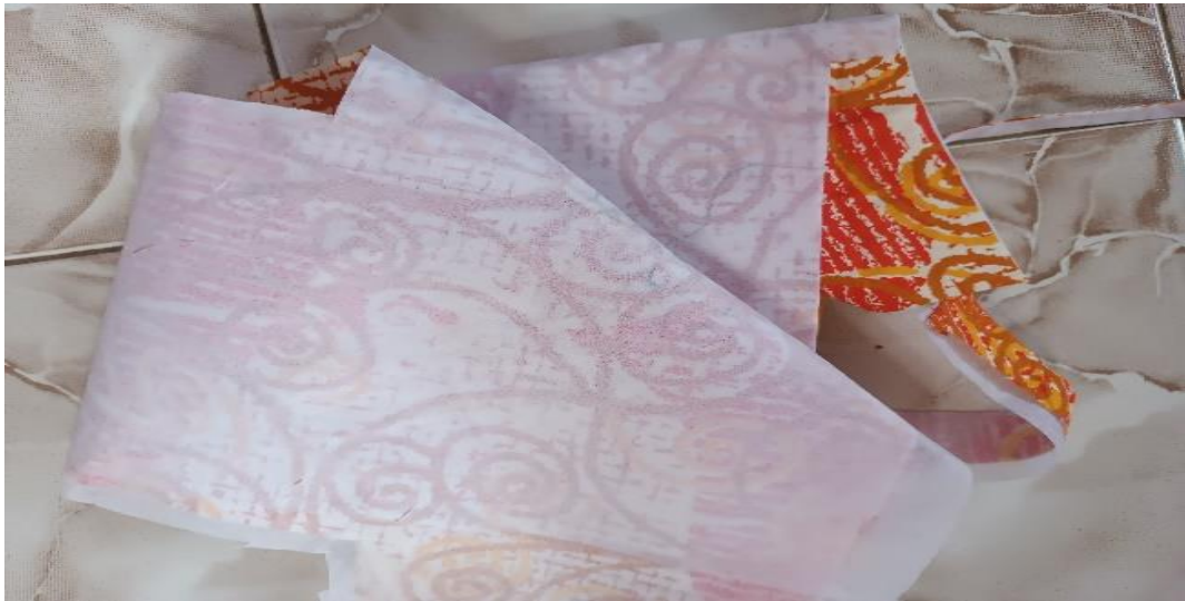
Figure 9: the gum-stay has been attached to the fabric using an iron. Source: Chudi-Duru (2026).
