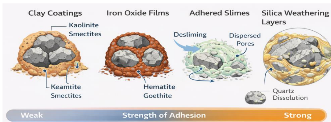
Figure 4. Mineralogical factors controlling attrition scrubbing efficiency. Adapted from Wills and Finch (2016); Sahoo et al. (2021); Wang et al. (2022); Gerber and Grobler (2023); and Mweene et al. (2024).
