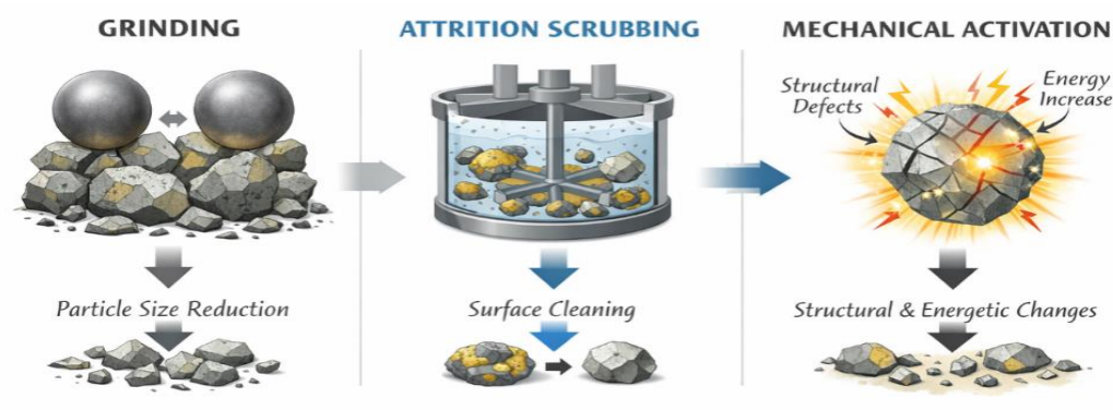
Figure 1. Conceptual comparison between grinding, attrition scrubbing, and mechanical activation. Adapted from Wills and Finch (2016); Wang et al. (2021); Sahoo et al. (2021); and Pereira (2026a).
