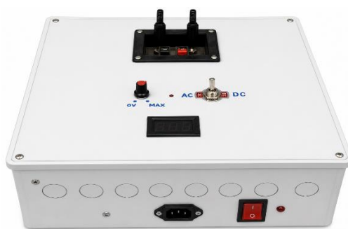
Figure 5: The Constructed Variable AC and DC Power Supply System
